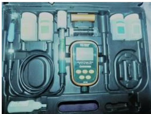
Plate 2.2: ExTech In-situ Water Kit for Measuring 7 Parameters
