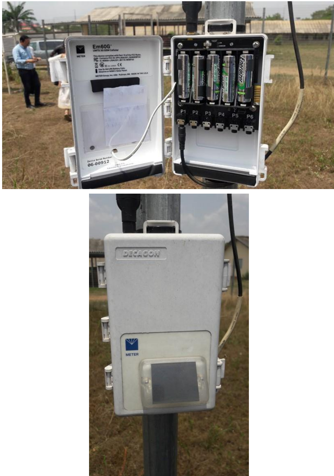
Plate 9: Automatic weather monitoring device of NIMET installed at observatory site of University of Ibadan (top-open and bottom-closed view)
