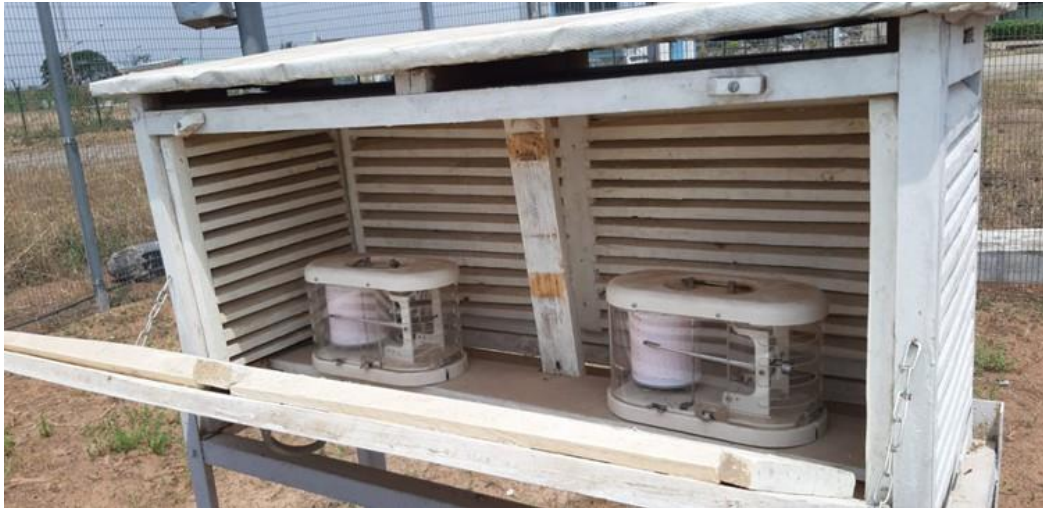
Plate 3: Weekly auto recording device for temperature and pressure at New Airport Observatory
