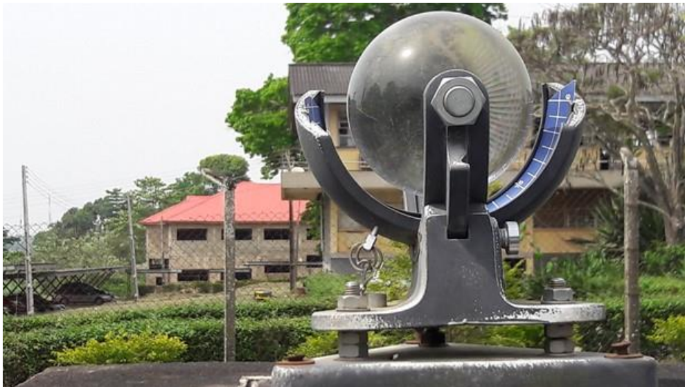
Plate 13: Sunshine hour device installed at Observatory site of CRIN in Ibadan
